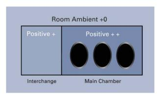
The Isolator main chamber pressure is positive to the room. The main chamber is slightly more positive than the pass-through interchange to ensure aseptic conditions within the main chamber.
